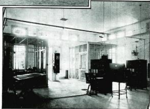
Screened measuring booths, precision clock, and high frequency receivers. The signal energy is transmitted to the measuring apparatus within the screened booths by means of a conductor enclosed in metal tubing.
