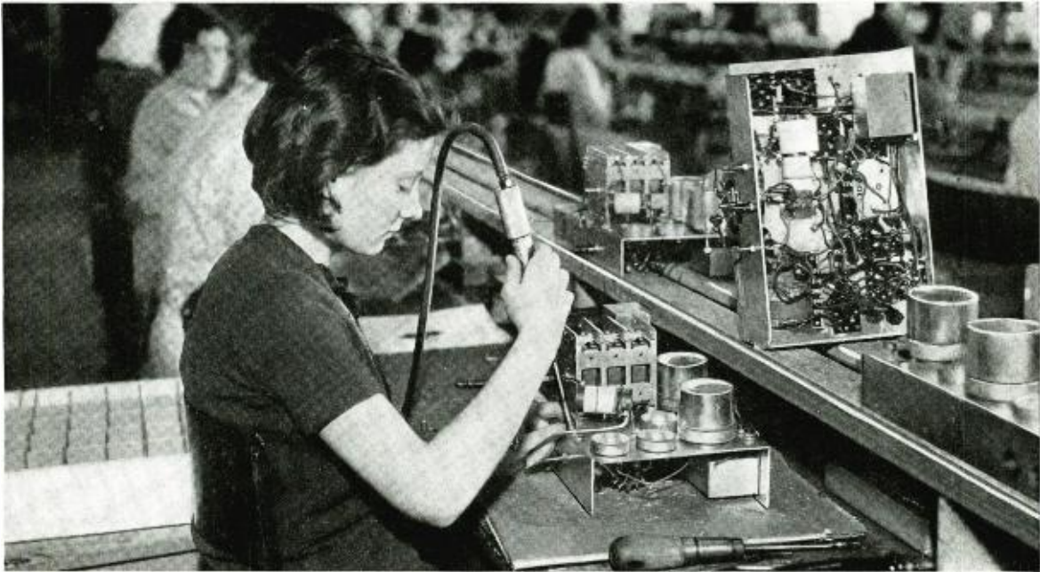
On the Pilot assembly line they speedily run in Self-tapping Screws with pneumatic and electric screw drivers.
